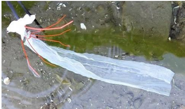
Figure 2: Plantee's bioplastic firm before being put in the St. Lawrence River for biodegradation testing
