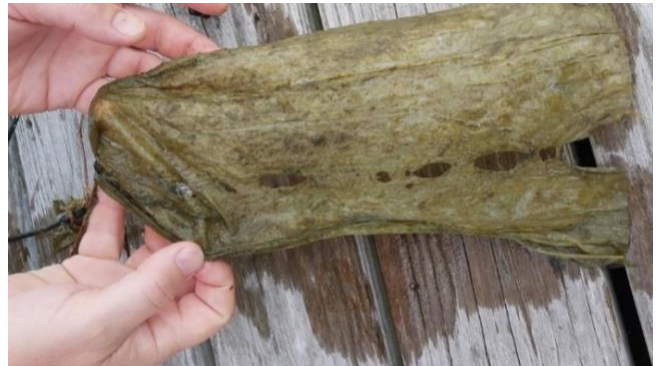
Figure 3: Plantee's bioplastic firm after 4 months in the St. Lawrence River. Demonstrates clear signs of degradation and tearing
